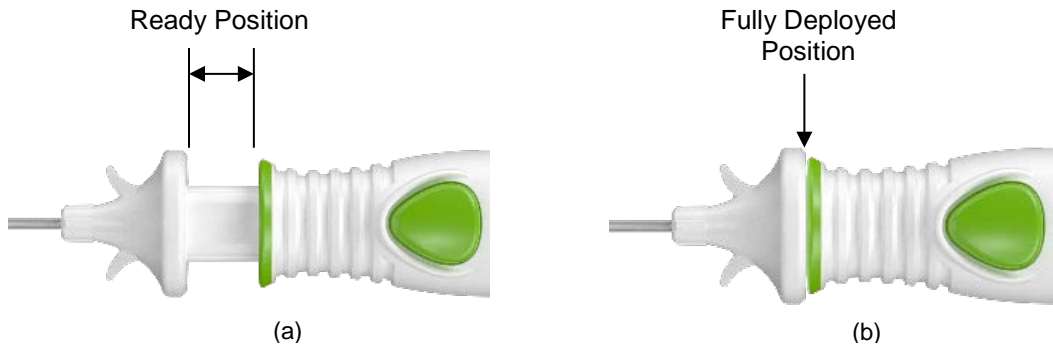
Figure 6: Images showing (a) Delivery Device Ready Position (b) Delivery Device Deployed Position
